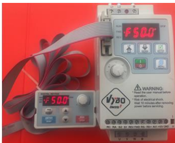
Connected external control panel
